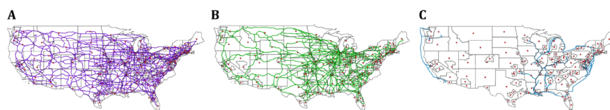
Figure 1. Real-world shortest path layouts between 129 FAF zones along the (A) highways, (B) railways, and (C) waterways within the U.S. Red points indicate the geographic centroid of each FAF zone. We convert the mode-specific infrastructure shapefiles into a graph of 129 nodes and 129 \times 128 shortest paths to be included in our multiobjective optimization model.
